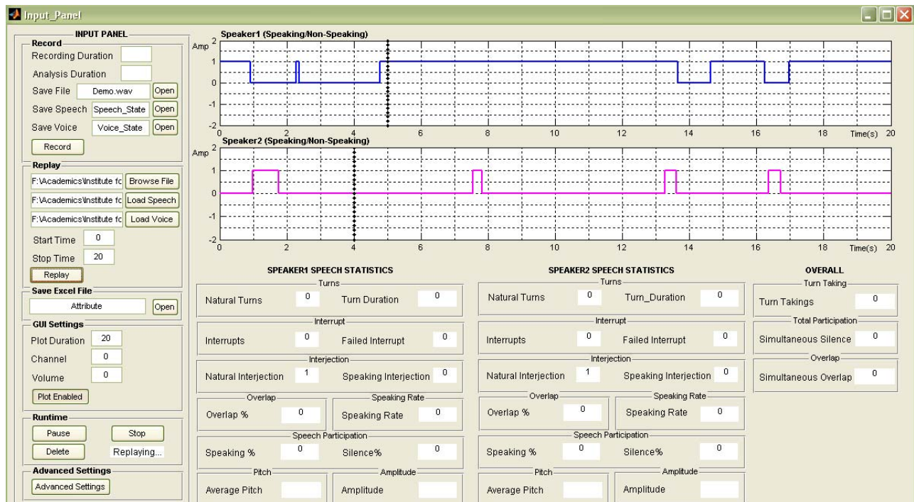
Figure 4. The Graphical User Interface (GUI) displays the speaker segmentation, and below those plots various non-verbal speech measures are displayed. On the left hand side, user Input Panel is at the top and controls panel is beneath it. The Advances Settings Panel (see Fig. 5) allows the user to specify parameter values for voice activity detection and speaker segmentation.
