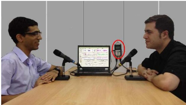
Figure 2. Recording system consisting of the Zoom H4n voice recorder (circled in red) and two Sennheiser e845s microphones, one for each participant in the conversation. The laptop can run the GUI (cf. Section III.C), which can be used to provide real-time non-verbal speech statistics to an external observer.
